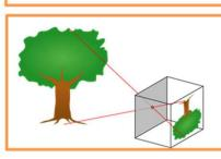
A pin hole produces an inverted image that be formed on a screen
